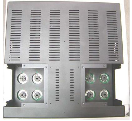
5. Insert the output tubes into each of the output tube sockets from tube # 1 to # 4 on the left side of the cover and 5 to 8 on the right side of the cover.
